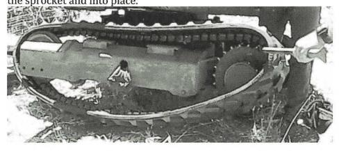
Note: If an additional person is available the track can be rotated in reverse to roll the track onto the sprocket.
