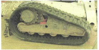
5. Using a 6' pry bar. Lift the front of the track and slide the inside portion of the track onto the front idler up to the track inner cleats.
