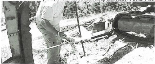
30. Tighten track adjuster relief valve.
