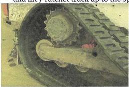
3. Push replacement track onto the sprocket and push lower portion of track into place under the rear idler.
